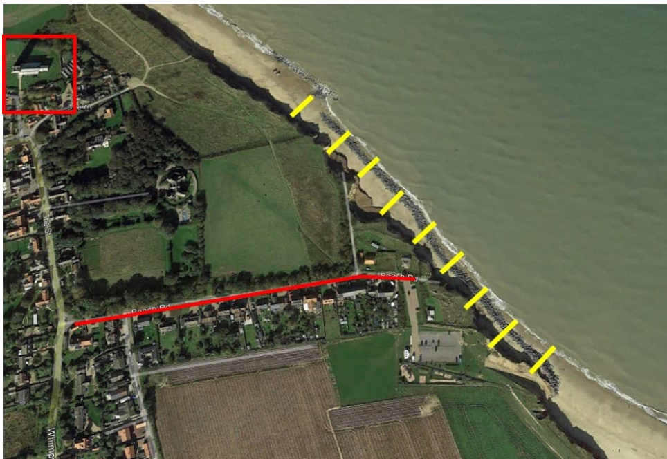
Figure 6-3. Illustration of potential rock groyne defences (yellow) at Happisburgh
