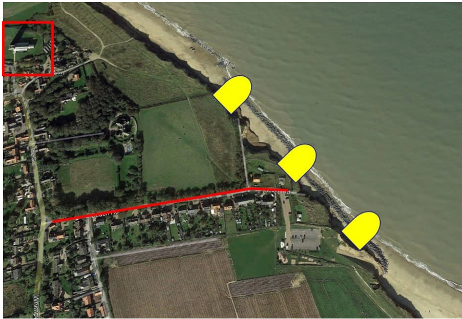
Figure 6-5. Illustration of potential rock headlands (yellow) at Happisburgh
