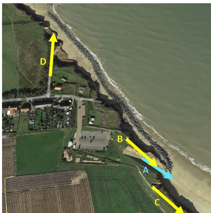
Figure 7-5 Shore-parallel ramp options at Happisburgh (yellow arrows indicate ramp slope top to bottom)
