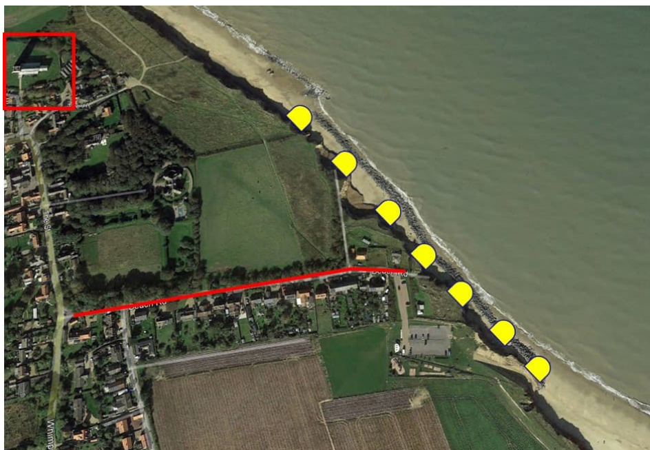
Figure 6-6. Illustration of potential rock bastions (yellow) at Happisburgh
