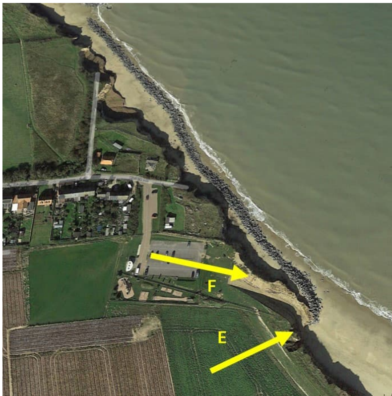
Figure 7-6 Shore-normal ramp options at Happisburgh (yellow arrows indicate ramp slope top to bottom)
