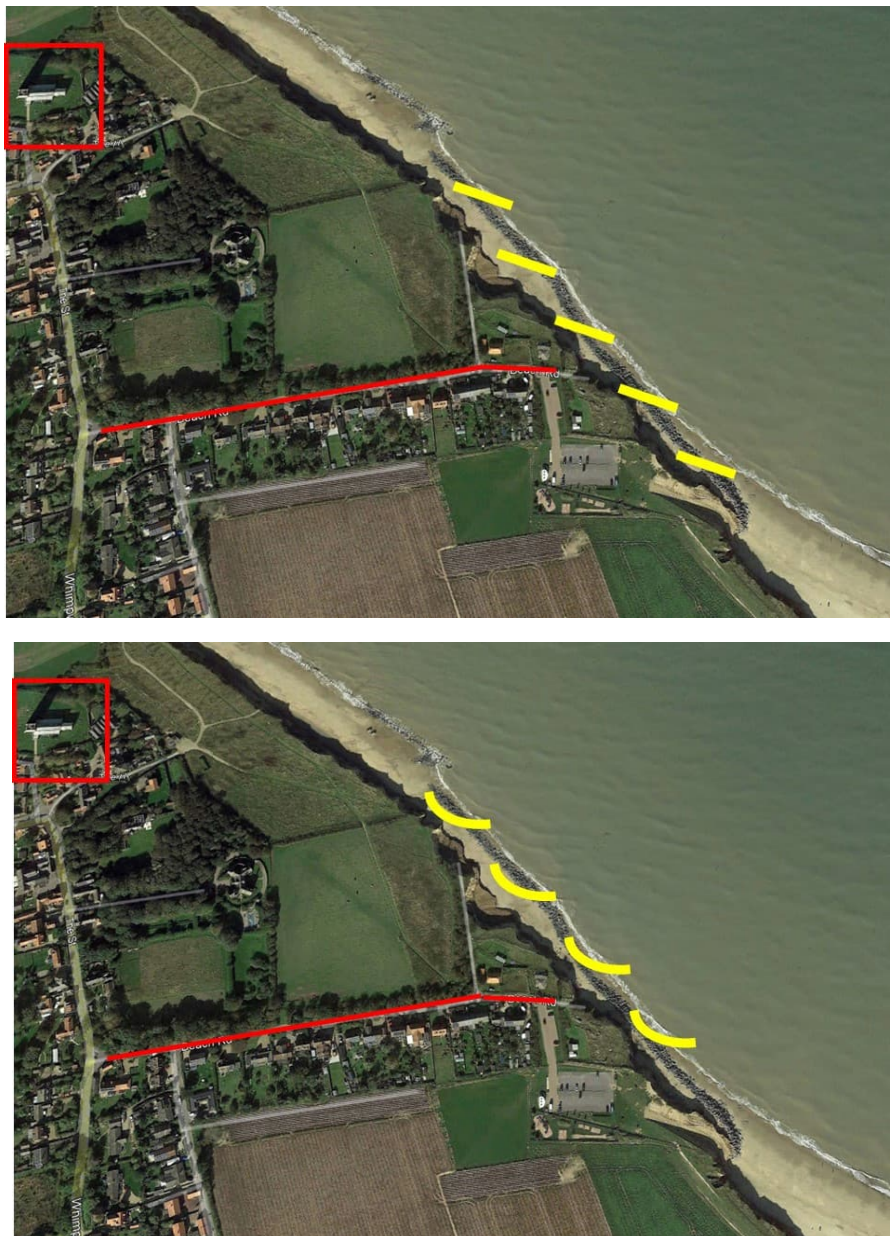
Figure 6-4. Illustrations of potential rock breakwaters (yellow) at Happisburgh
