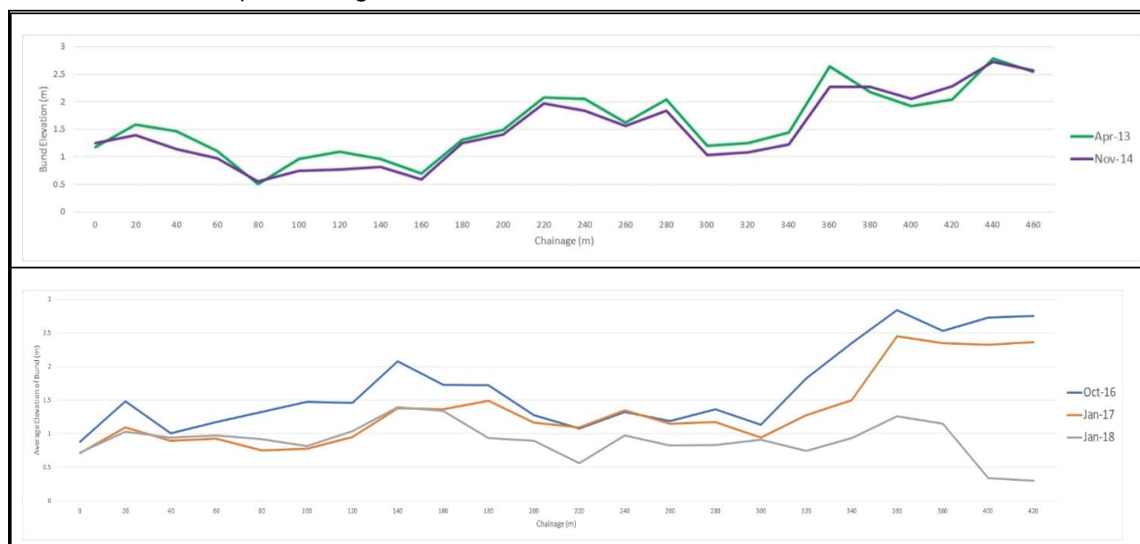
Figure 3-7. Rock Bund Crest Elevation (upper graph shows first configuration of bund post-2013, lower graph shows second configuration of bund between 2015 and 2018)
