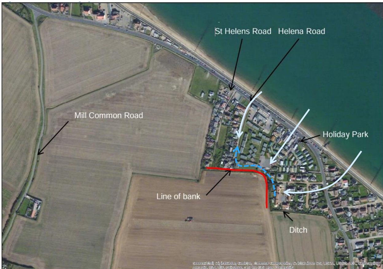
Figure 2-1: Locations of flooding in Walcott (light blue line) and the embankment (red line) which prevented water entering the field system behind, routing water along the blue-dotted line.
