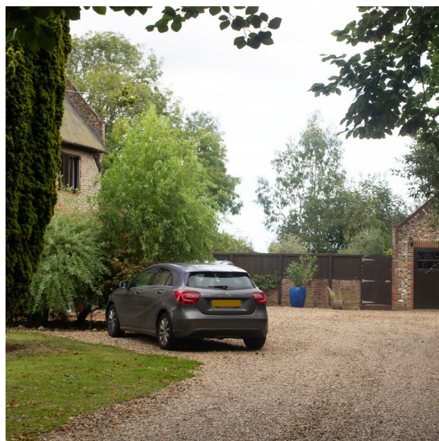
Figure 19: Positive example of car parking with a permeable gravel surface, reducing surface water runoff.
