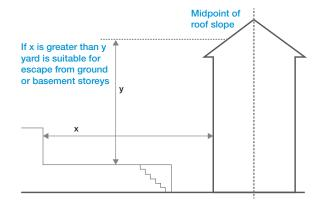
Where provided for escape from a room above ground storey level, a dormer window or roof light should be positioned as indicated below:
