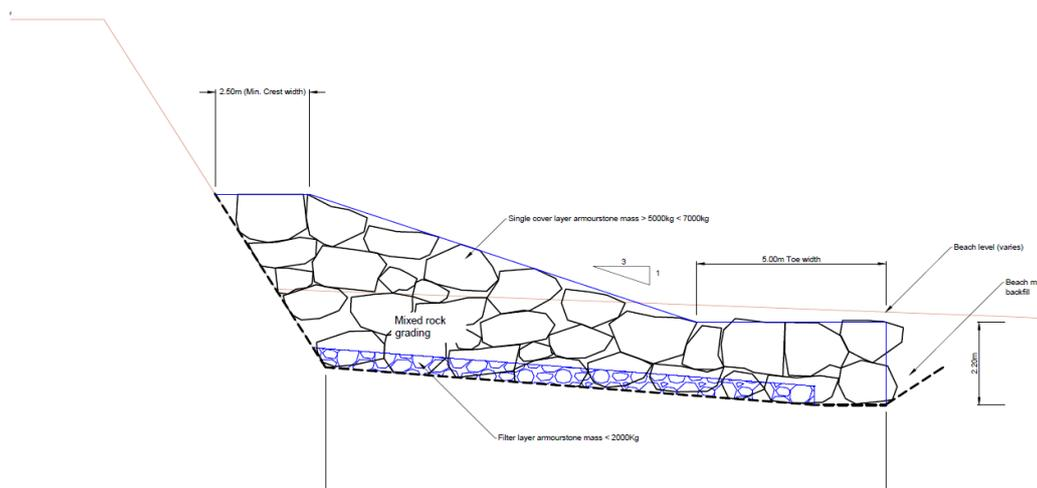
Figure 3. Cross section through rock revetment
