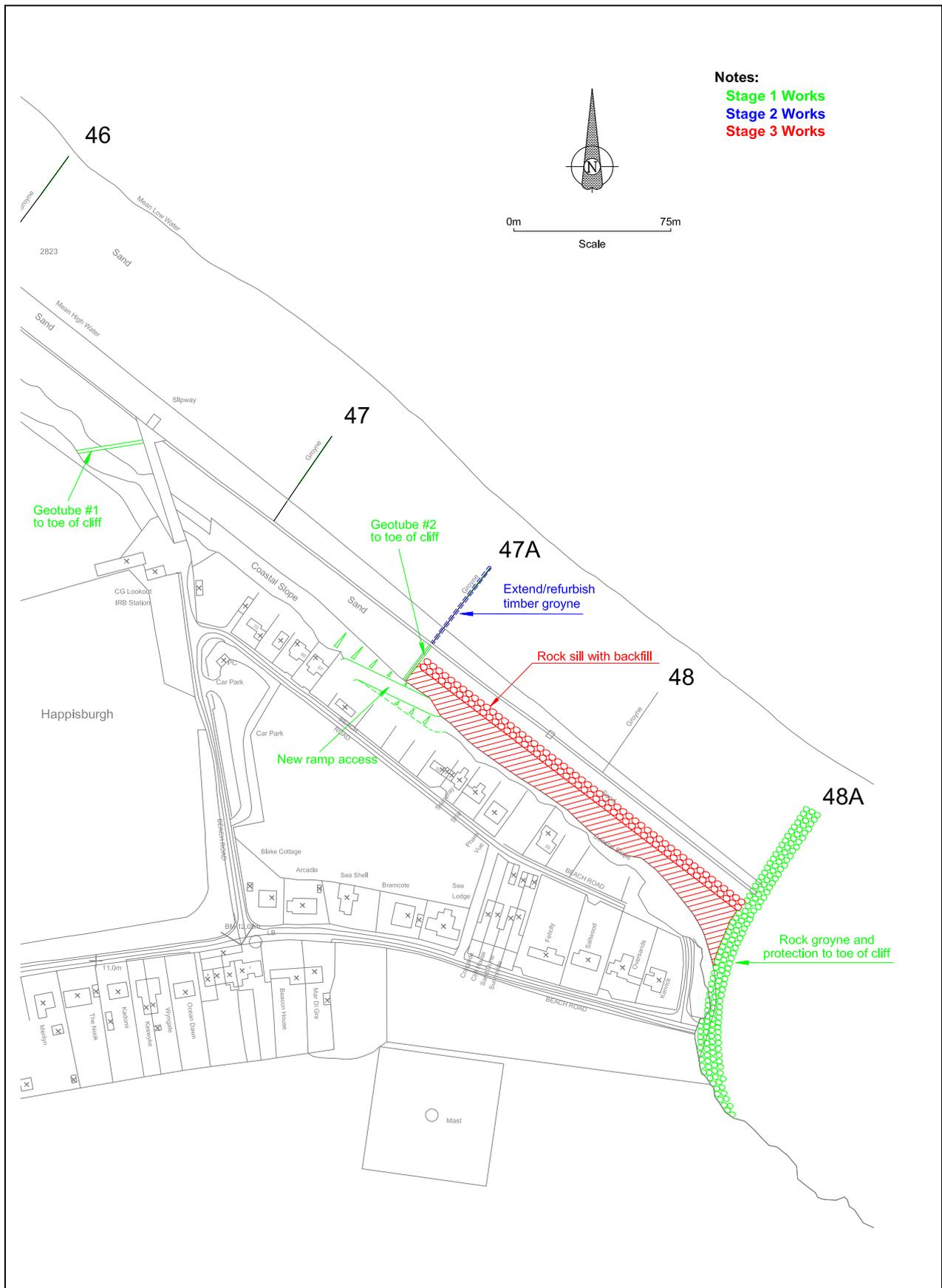
**Figure 9 General arrangement of defence works**
