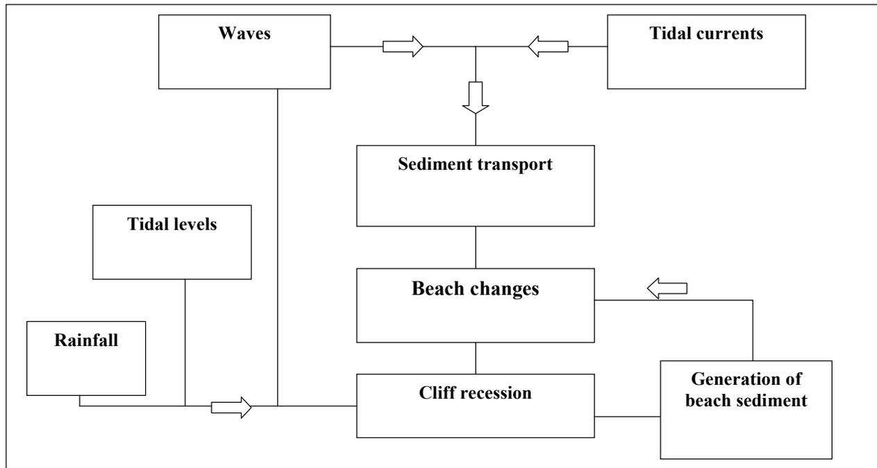
**Figure 4 Simplified flowchart of littoral processes**
