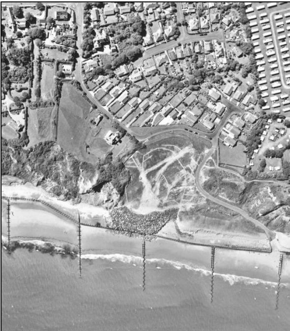
The top left photograph is shows Clifton way in 1986 before the major failure occurred. The top right photo is from 1994 and shows the extent of the failure at that time. The photo on the left was taken in 2000, approximately 5 years after the site was stabilised. The rock armour is clearly visable at the toe of the slide and many of the surface drains can also be seen.
