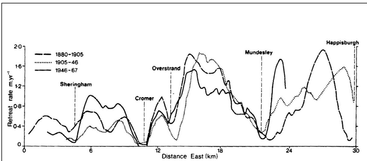
**Figure 1.1 Variation in cliff recession rates along the North Norfolk coast (Cambers 1976)**
