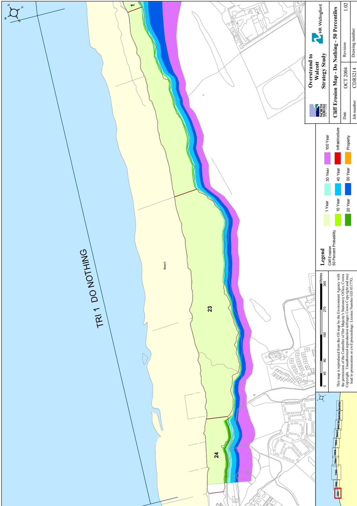
**Figure 2.1 Predicted cliff recession to 100 years. Do Nothing scenario TRI1**
