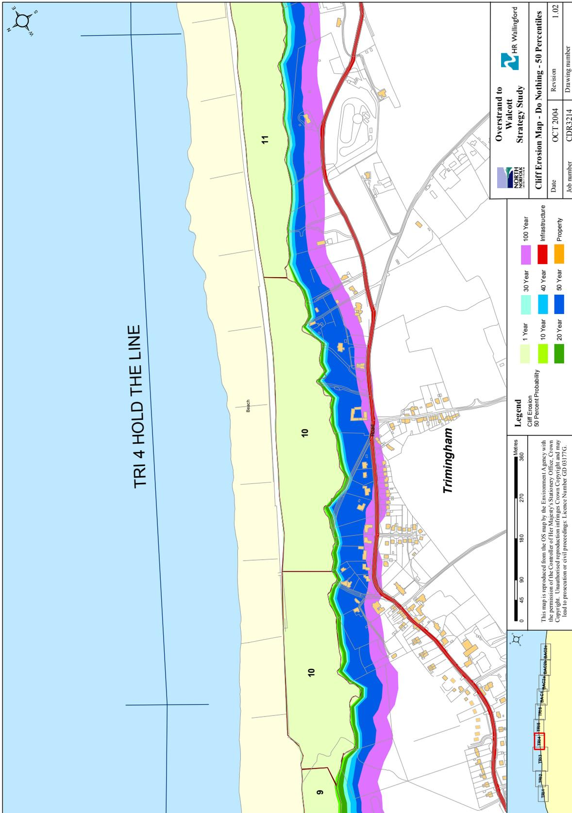
Figure 2.4 Predicted cliff recession to 100 years. Do Nothing scenario TRI4
