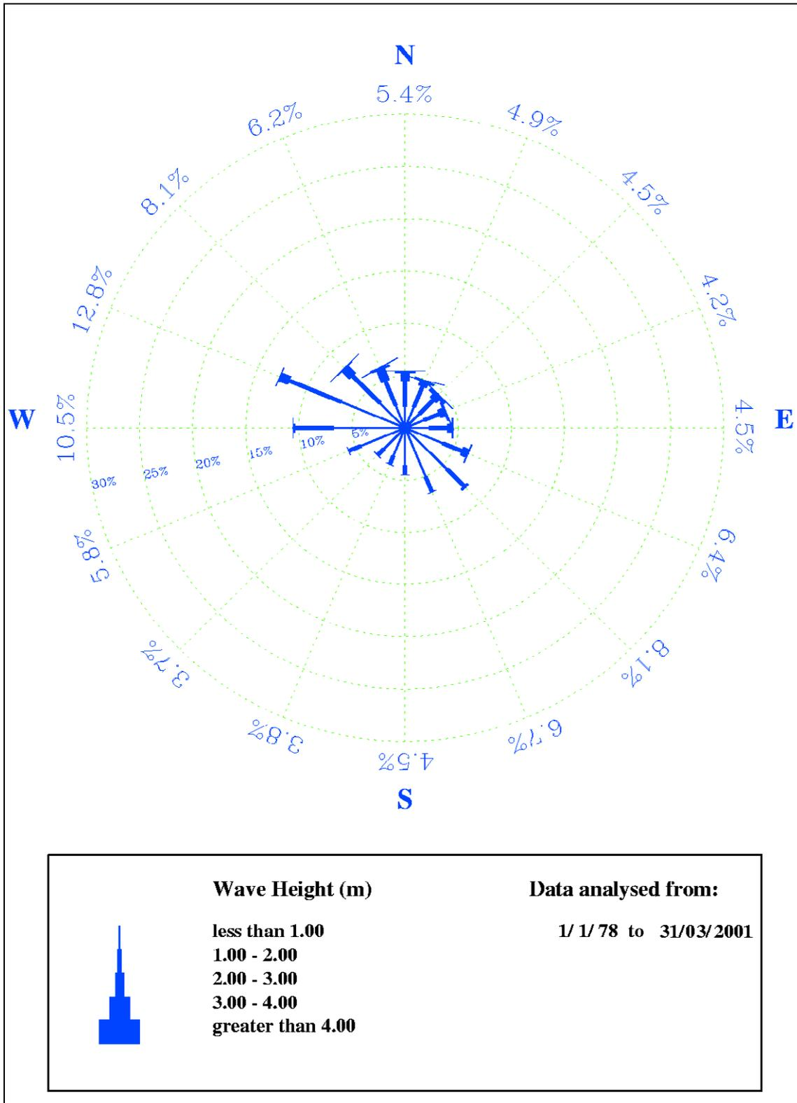
Figure 4.3 Wave rose showing offshore wave conditions
