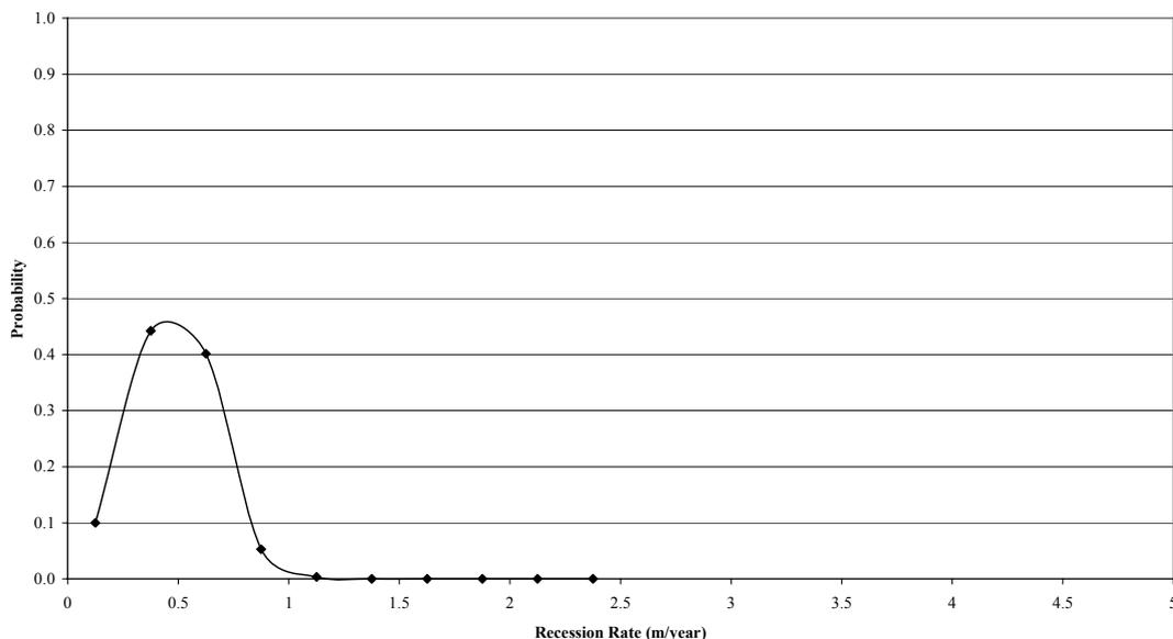
**Figure 20 N2A2-3 (Cliff Unit 2b): Recession Rate Probability**
