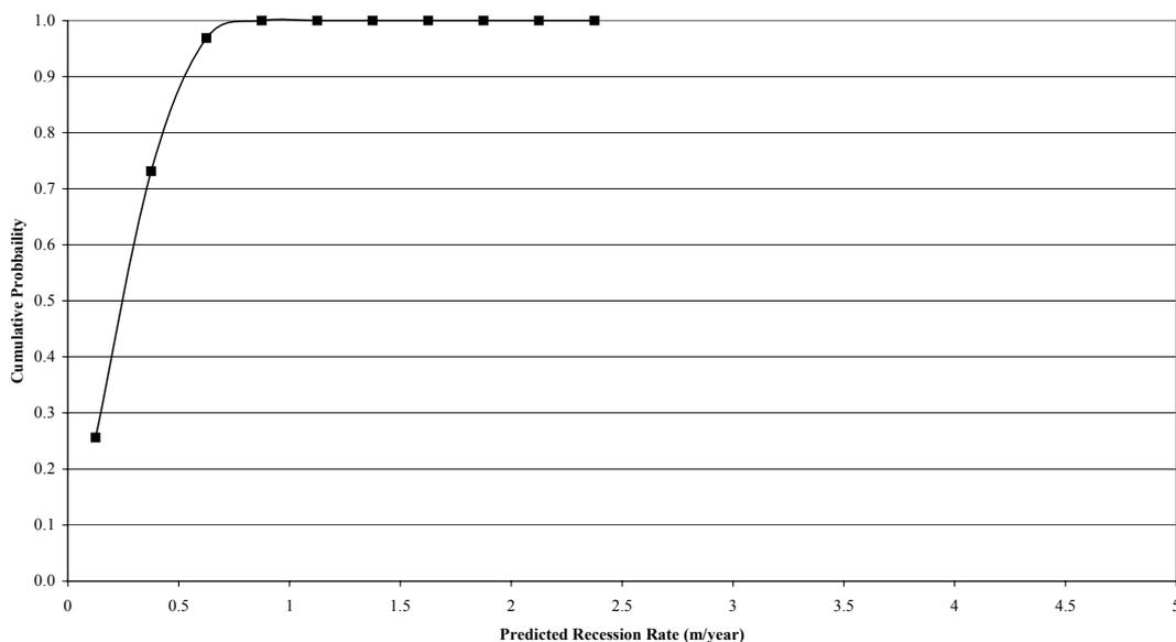
**Figure 16 N2E2-N2E3 (Cliff Unit 5b) Cumulative Probability: Annual Recession Rate (m/year)**
