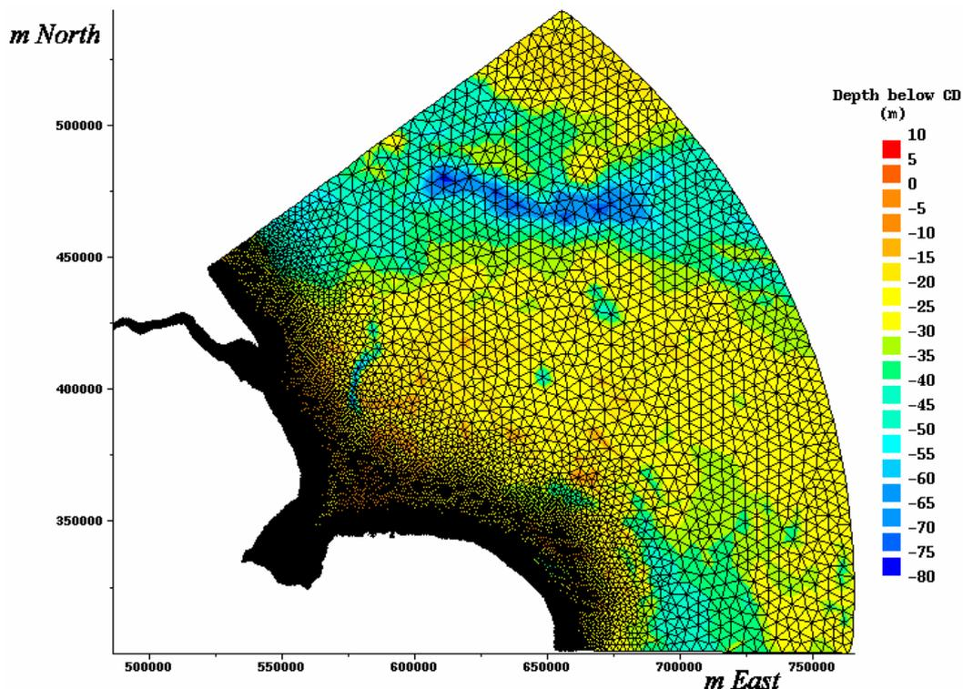
Figure 4.4 Bathymetric grid used for wave transformation modelling
