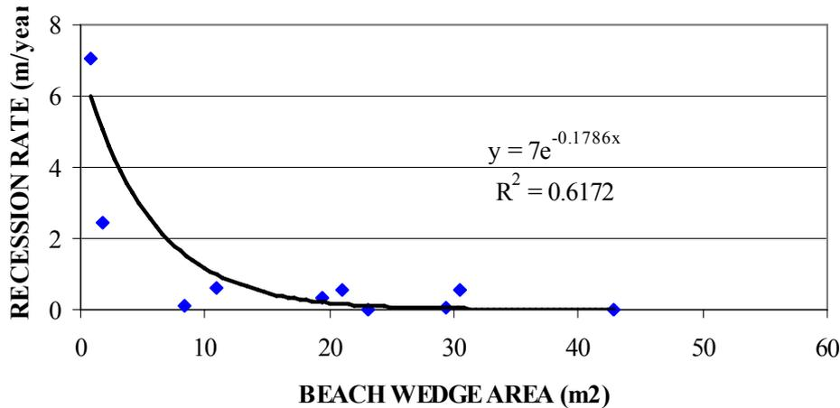
**Figure 5 Norfolk Cliffs: Recession Rate and Beach Volume (Unprotected)**
