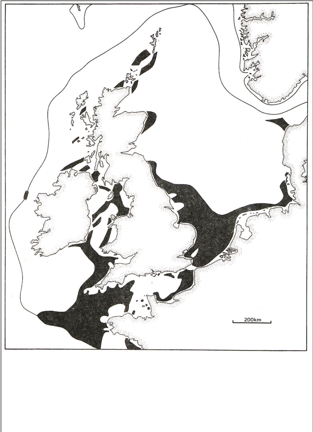
Figure 26 Distribution of sandwaves (dark shading) on the North West European continental shelf. Reproduced from Stride, 1982, with permission from Chapman and Hall
