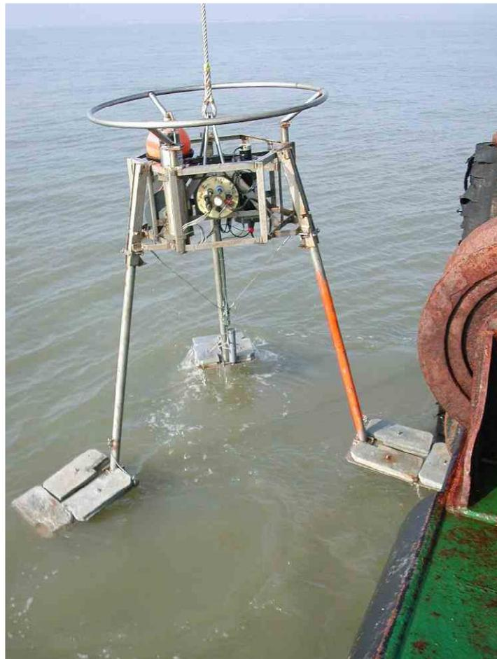
**Figure 4** CEFAS Minipod being deployed at Clacton
