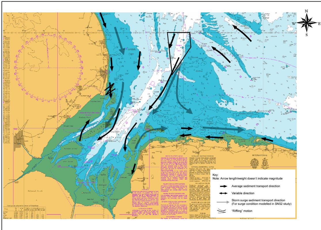
**Figure 3** Schematic sediment transport pathways for average conditions and interpreted for the extreme water level (surge), wind and wave event modelled in this study (overlain on Admiralty Chart 1408)
