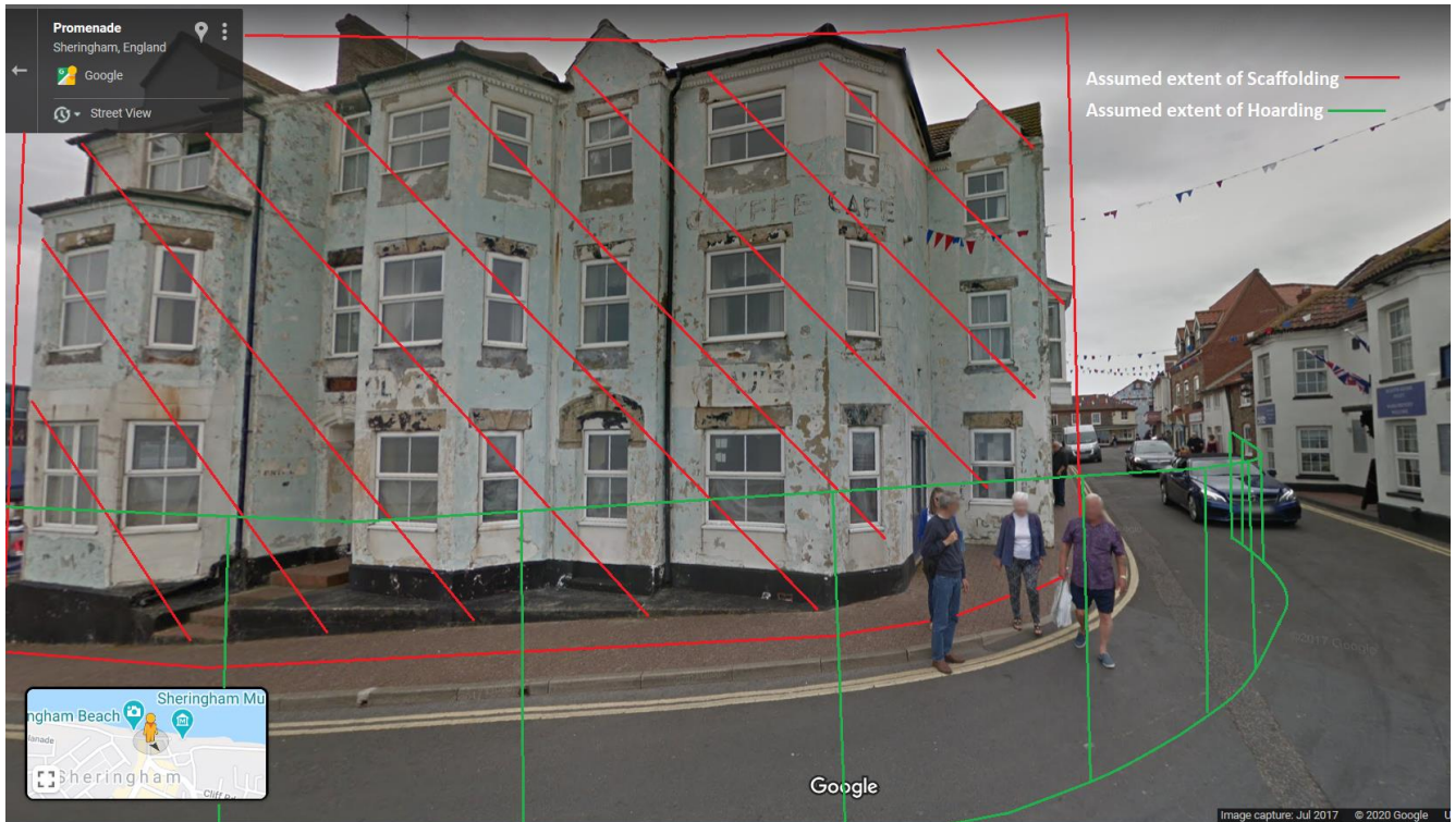
Figure 1. Rough depiction of the assumed extent of proposed scaffolding and fencing/hoarding, partially encroaching on High Street
