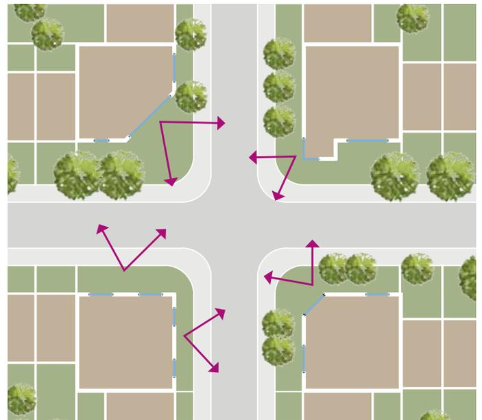
Figure 51: Diagram reflecting design principles for corner buildings.
