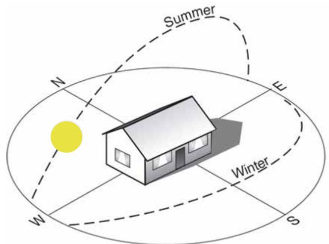
Figure 85: Illustration to show the appropriate building orientation so as to maximise solar gains. Windows should be placed mainly on the southern side whilst fewer openings should be located on the northern. A deep roof overhang can offer some shading. This can also be improved with some trees and vegetation around the house. (Source: <https://nextdayinspect.com/building-orientation-for-optimum-energy/>).
