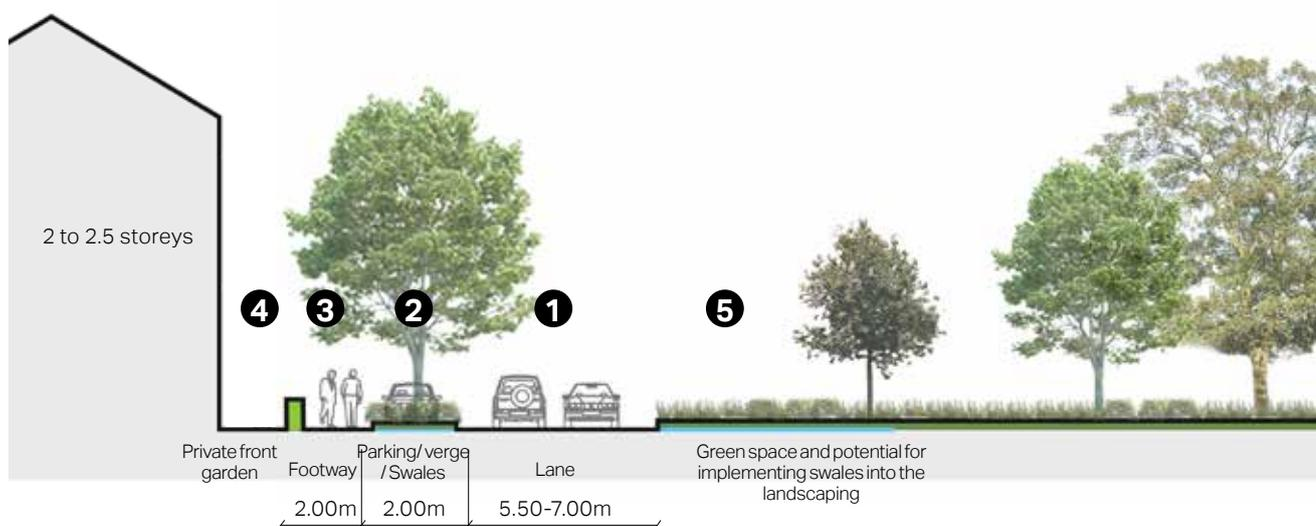
Figure 24: Section showing indicative dimensions for main entrances.
