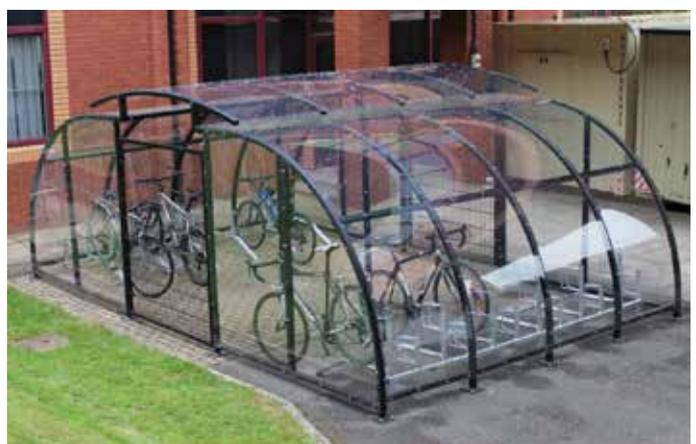
Figure 36: Example of a communal cycle parking in a residential scheme, UK.
