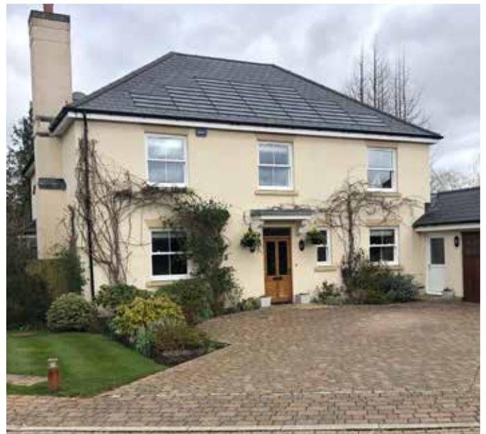
Figure 87: Use of shingle-like solar panels on a slate roof, with the design and colour of the solar panels matching those of the adjacent slate tiles in Lingfield, Surrey.
