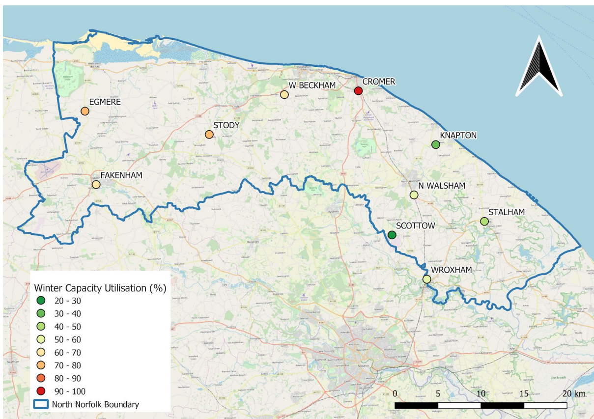
Figure 3: Winter capacity utilisation of 33kV substations in the North Norfolk area
