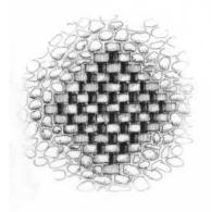
Honeycomb ventilation panel - can be fitted internally with inward opening casement window. Gives superb patterns of light and shade.
