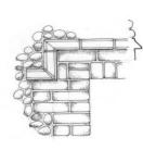
19th century drip mould using 'special' bricks.
