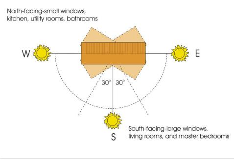
Figure 2 Principles of passive solar design
