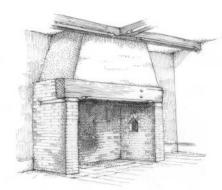
17th - 18th centuries. The so-called inglenook. There are infinite variations of detailing! Often combined with a domed bread oven, salt 'cupboards' and staircases to one side. Traces may still exist to tell their story.
