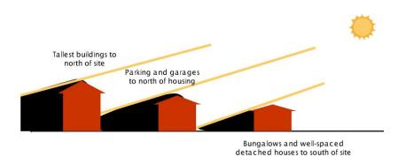
Figure 1 Planning to minimise overshadowing
